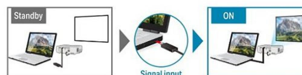
\*9 Supported terminal are COMPUTER IN 1, HDMI 2 and VIDEO. This function is unavailable when STANDBY MODE is set to WOL or SAVING. This function may work unintentionally by connected external device.
